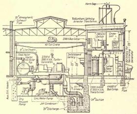
Fig. 242.—Arrangement of the generating and electrical equipment in a modern steam-turbine generating station.\*
